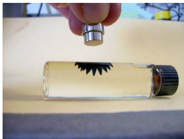
Fig. 7 Spike formation in a magnetic fluid under the influence of a permanent magnet
